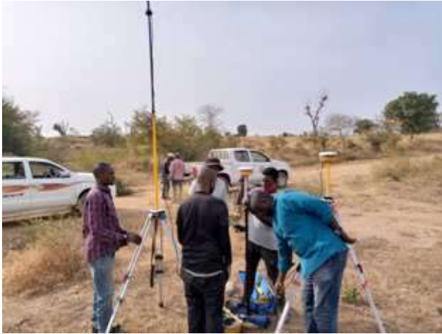
Survey unit at work with V30 Hi-Target Differential GPS at Jimere- Yola Nora
