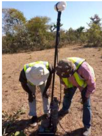
Magnetic surveys with GSMP-25 WALK Magnetometer
