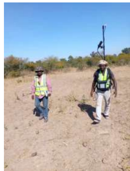
Magnetic surveys with GSMP-25 WALK Magnetometer
