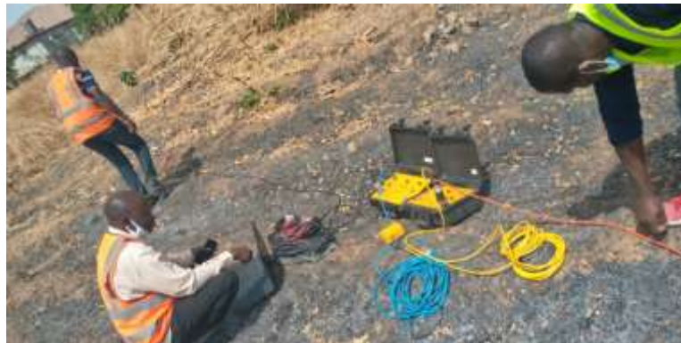
48 Channels Seismic Equipment being used for Foundation Studies
