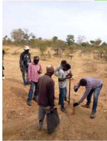
Survey unit at work with V30 Hi-Target Differential GPS at Jimere- Yola Nora
