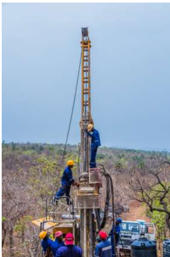
HYDX – 6 Crawler Mounted Drilling Rig in operation at Tajimi Iron Resource, Kogi State State
